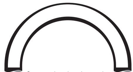
Compression along inner edge. Thinning along outer edge.
